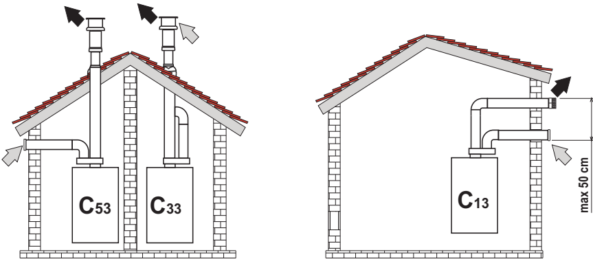
fig. 25- Examples of connection with separate pipes
